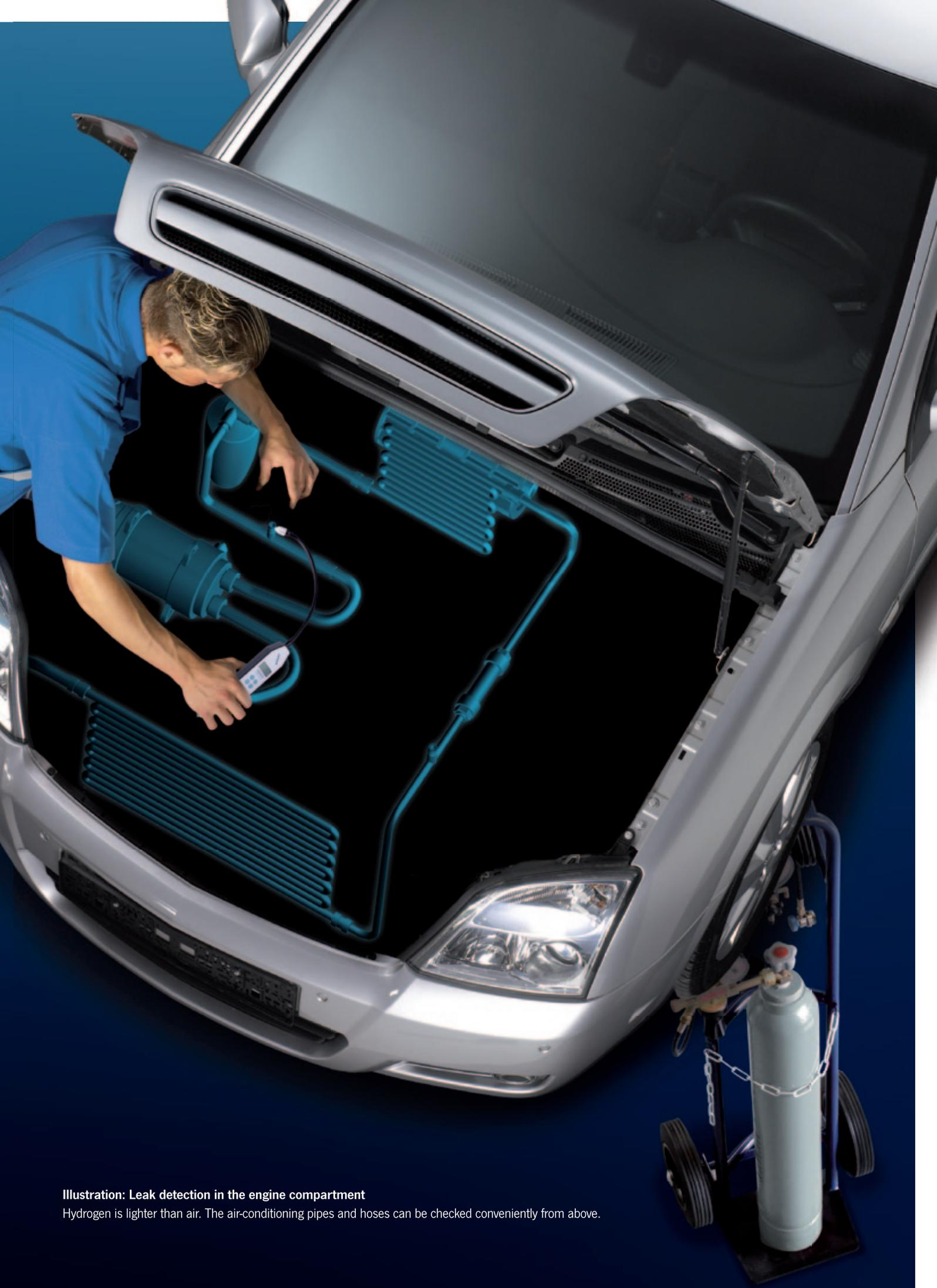
**Illustration: Leak detection in the engine compartment**
